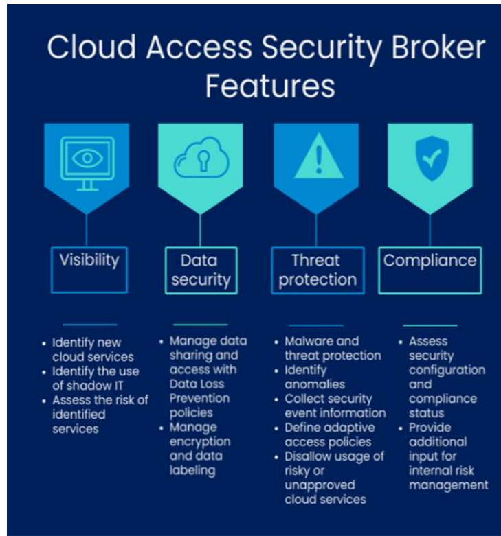
Figure 4: Cloud Access Security Broker (CASB) Features [42]
